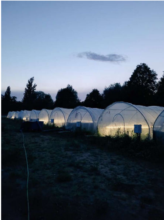
Exterior view of the Riparian Stream mesocosms (RSM) in Landau, Germany (RPTU Kaiserslautern-Landau, RTG SystemLink). The facility consists of replicated outdoor artificial stream channels designed for controlled experiments on riparian and stream ecosystems. During this experiment, selected stream channels were illuminated at night with artificial light at night (ALAN), whereas others remained dark and served as controls. (Photo by Alessandro Manfrin).
