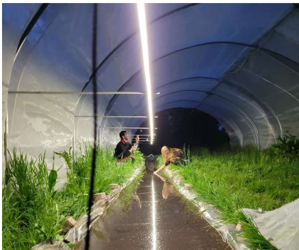
Interior view of the Riparian Stream mesocosms (RSM) in Landau, Germany (RPTU Kaiserslautern-Landau, RTG SystemLink). Each mesocosm consisted of an artificial stream channel surrounded by riparian habitat, supporting natural communities of aquatic insects, riparian vegetation, and terrestrial arthropods, including spiders. Half of the mesocosms were illuminated during nighttime, while the remaining mesocosms maintained under dark control conditions (photo by Alessandro Manfrin).
